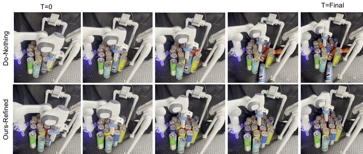
Fig. 5: Method comparison in Real robot experiment. The first row shows the Do-Nothing baseline on the real robot, where the end-effector directly pushes through the clutter, resulting in object being knocked over. The second row shows our refined model, which enables controlled contact and safely navigates through the dense environment. The comparison demonstrates how the refined model allows for contact while preserving safety in real-world settings.
